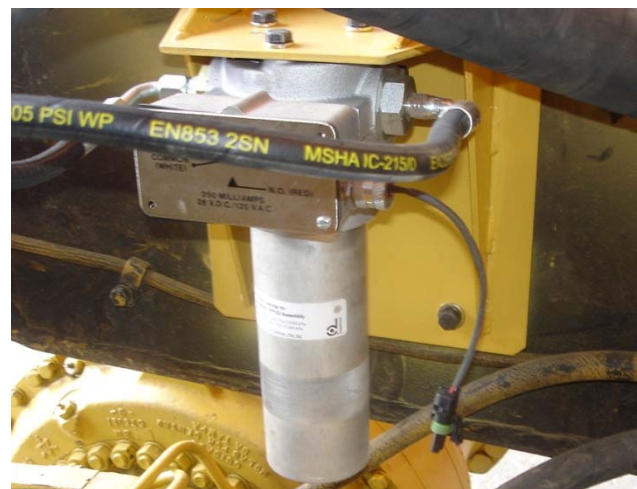
Figure 1.00 – Pilot Line Filter Assembly
